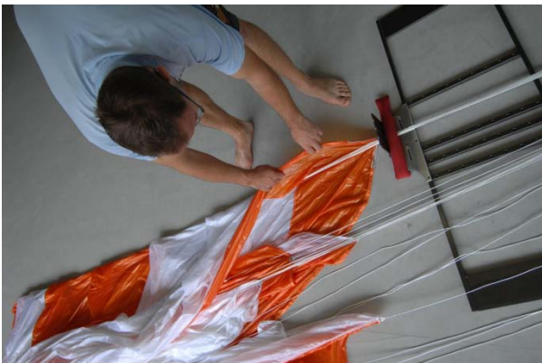
Fig. 30 pick up the trailing edge starting at the middle line
