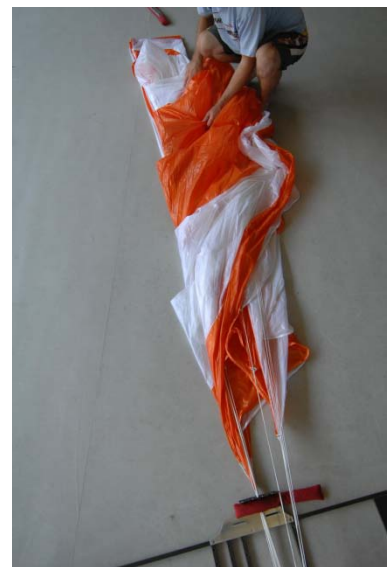
Fig. 63-64 put opposite half of the wing including lines over the line separator to the other side
