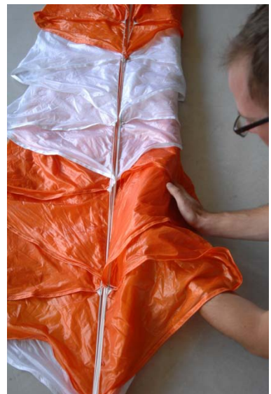
Fig. 70 all the lines have to be on top of the sail in the middle
