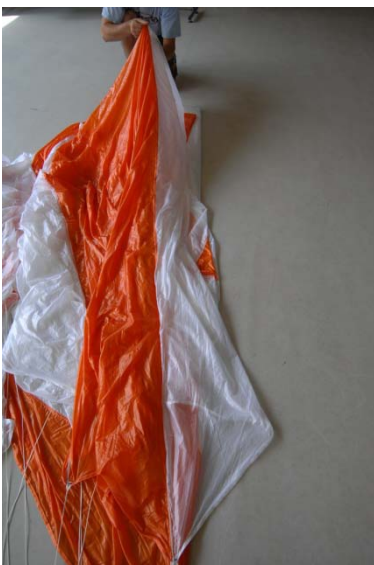
Fig. 41 pull out panel No. 3
