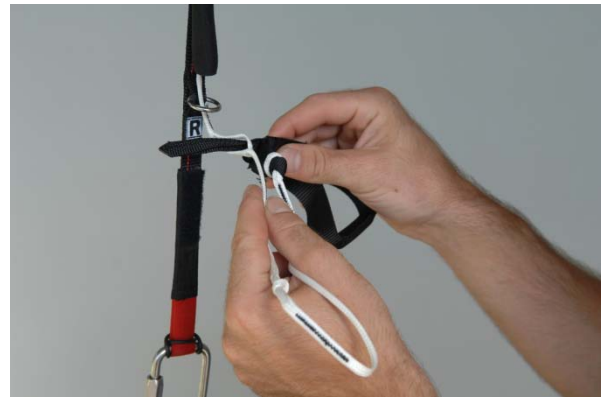
Fig. 4 Stowing the brake line for opening with brakes applied. Shoulder attachment of the reserve parachute.
