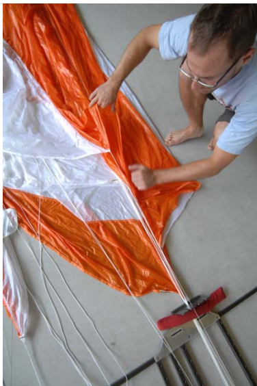
Fig. 50 anchor the line of panel No. 5 to the line separator
