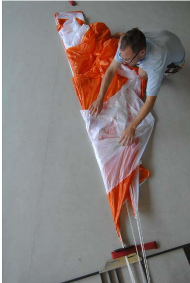
Fig. 65 the middle lines form the axis of symmetry
