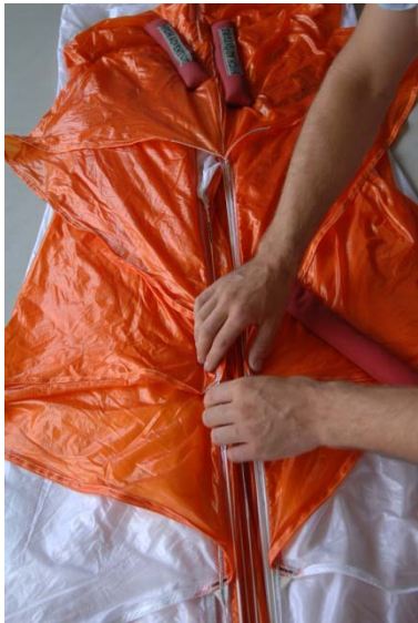
Fig. 68 check free run of the lines...
