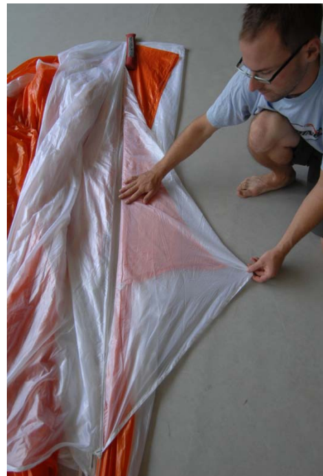
Fig. 37 lay the second panel on top of the first
