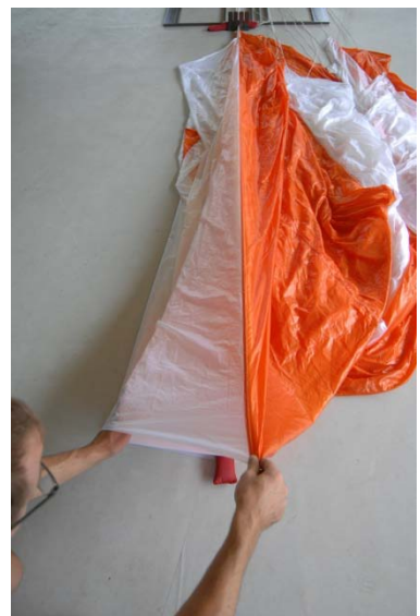
Fig. 43 put it on top of panel No. 2 (applying slight tension)
