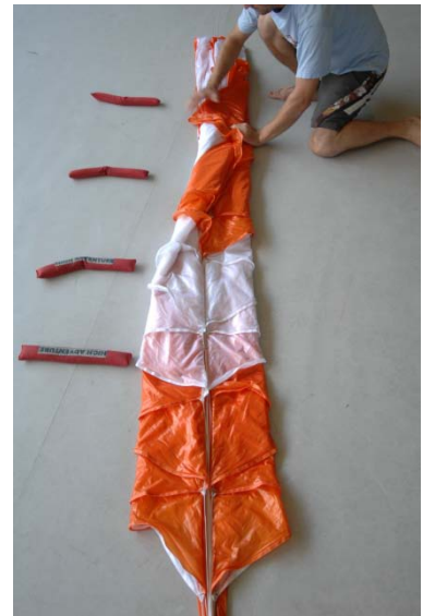
Fig. 79 Put wing sides on top of each other
