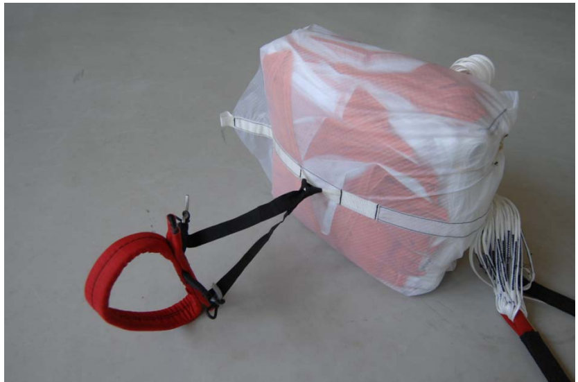
Fig. 112 Attachment of handle when using front container
