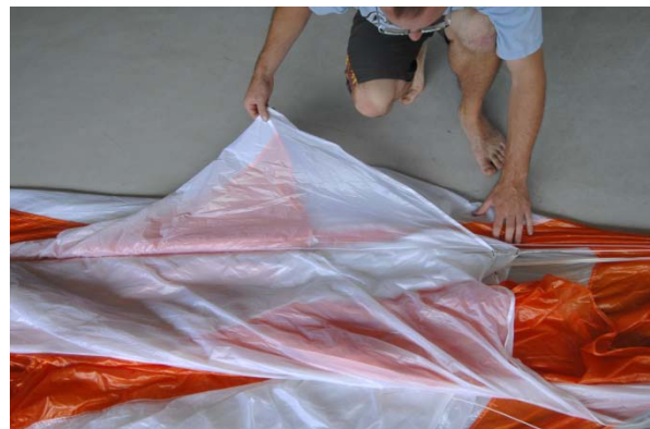
Fig. 35 anchor the line from Panel No. 2 to the line separator
