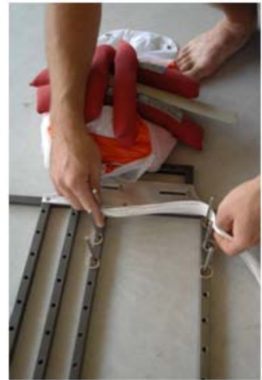
Fig. 99 place the suspension lines in figure eights... (pay attention that the width of the inner container is not exceeded)
