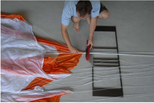
Fig. 32 fasten the line of panel No. 1 in the line separator. Fig. 33 spread out panel No. 1. Caution: make sure that the line is on top of the middle lines, which forms the axis of the reserve. Shape and size of this panel can vary depending on the brake configuration.
