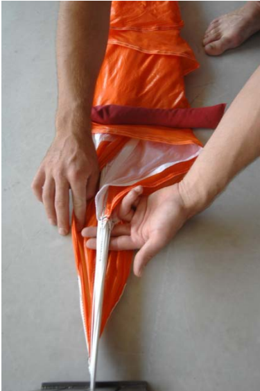
Fig. 82-84 wrap panel No. 1 around all the lines...
