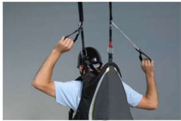
Fig. 2 Attached to the dedicated reserve bridle attachment points of the harness (shoulder attachment)
