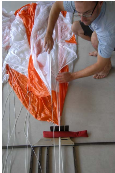
Fig. 39-40 anchor panel No. 3 in the line separator and put the line with its attachment point of panel No. 3 on top of the middle lines
