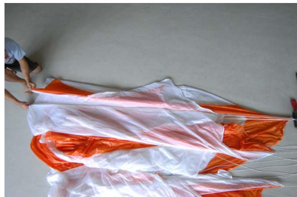
Fig. 34 reduce panel No. 1 using a double s-fold
