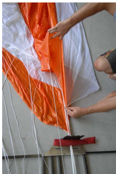
Fig. 45-46 anchor the line of panel No. 4 to the line separator
