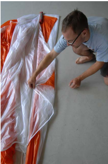
Fig. 38 reduce panel No. 2 by s-fold
