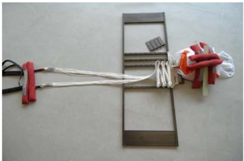
Fig. 101 the last 50-60cm of the suspension lines are used to close the container and must remain free from rubber bands.
