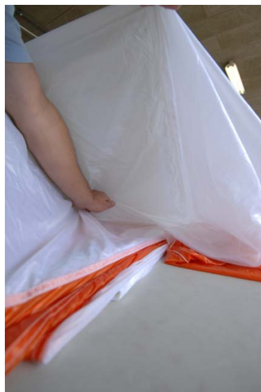
Fig. 42 sweep panel No. 3 outwards (s-fold)
