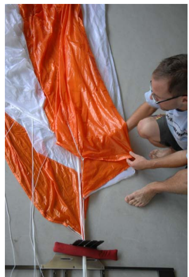
Fig. 45-46 anchor the line of panel No. 4 to the line separator
