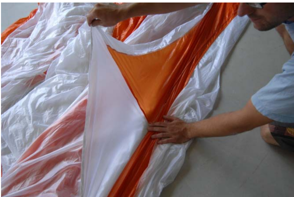
Fig. 36 put the line with its attachment point of panel No. 2 on top of the middle lines and fix it with your hand
