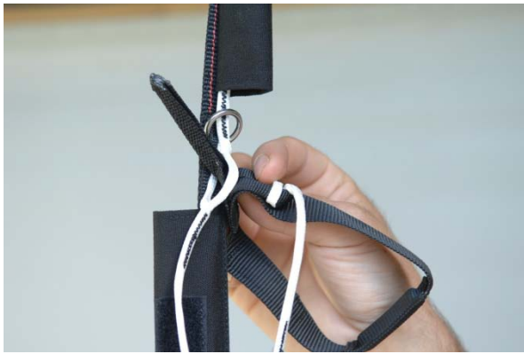
Fig. 3 Stowing the brake line for opening with brakes applied. Front attachment of the reserve parachute.
