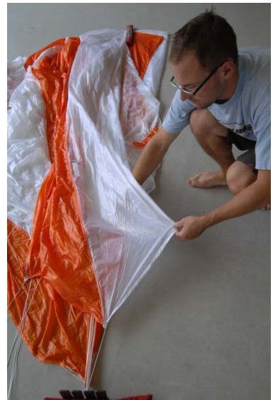
Fig. 39-40 anchor panel No. 3 in the line separator and put the line with its attachment point of panel No. 3 on top of the middle lines
