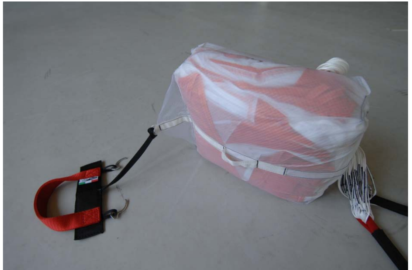
Fig. 108 Attachment of handle when using integrated container.
