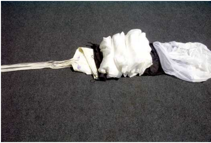
21. Put the canopy in small "S"-foldings in front of the container.
