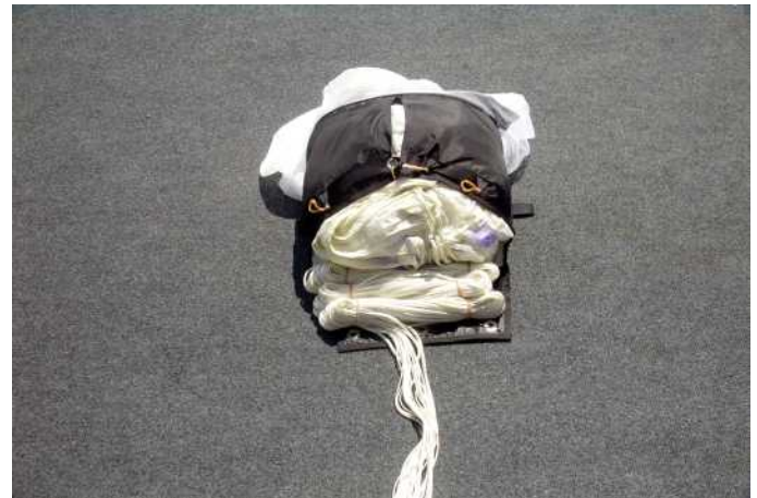
24. The rest of the canopy's base is put in "S"-foldings into the container. Also the line bundles are put in the container.
