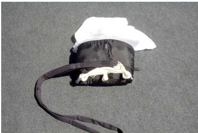
25. Close the inner container with the last 50cm of the lines. First close the centre, than the sides.
