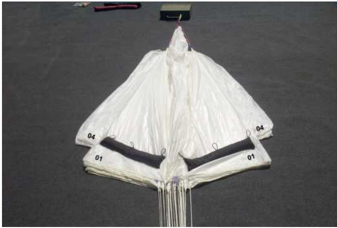
15. In the middle there is one between-segment left over now. This segment is smoothed upward and put between the segments No.01.
