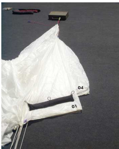
9. Put all further segments until segment No.1 on each other. Fix the segments with a packing-weight
