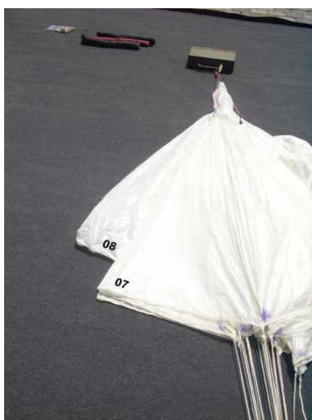
12. Put segment No.07 on segment No.08 until the between-segment No.04 appears.
