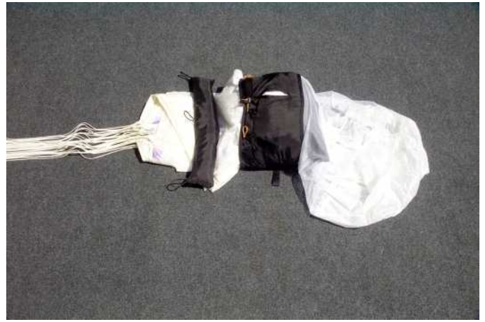
22. Put the "S"-folded canopy in the inner container now.
