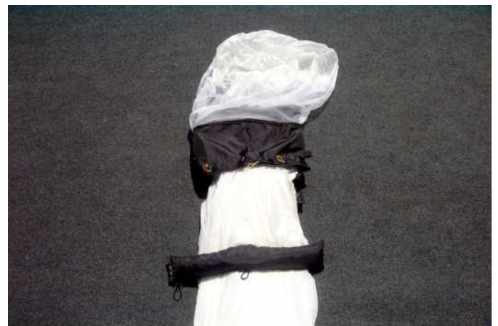
20. Put the upper end of the canopy in the inner container.
