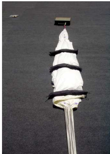
17. Fold the canopy in form of a "S". Approximate 1/3 of the right side is put under the lines.
