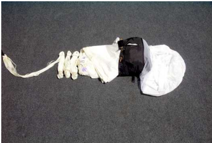
23. About 30 cm of the canopy's base are still outside the container. Bring the lines in 3x3 bundles in form of a "8".
