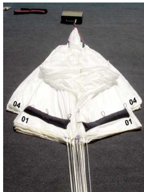
14. Put the further segments over each other and fix it with a packing-weight.
