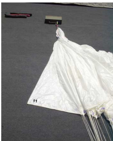
10. Attach the apex of segment No.11 (left side!) into the third packing-cord and pull segment No.11 to the side.
