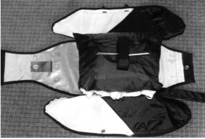
11. The bridle is placed in an "S" shape on the base of the outer container. Arrange the bridle so that it comes from the outer container on the left or right side, depending on the needs of the pilot.
