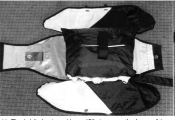
11. The bridle is placed in an "S" shape on the base of the 12. At first close the side flaps. outer container. Arrange the bridle so that it comes from the outer container on the left or right side, depending on the needs of the pilot.
