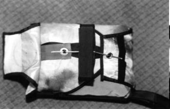
13. Finish by closing the lower fastening flap and finally the 14. To avoid an unintentional opening the DHV prescribe to covering flap.
