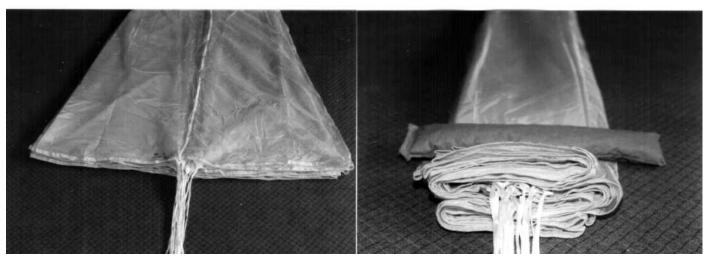
3. The canopy is placed on the table and folded such that 4. Fold the canopy in the form of an "S", so that the lines are the stamped segment (No. 1) lies on the top.
