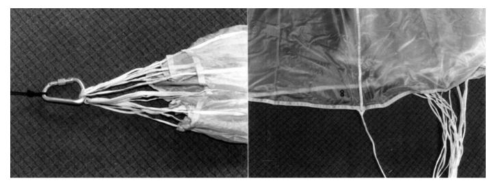
1. Secure the parachute at its apex to a suitable hook.
