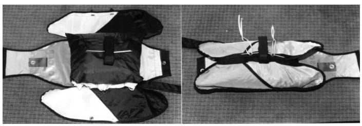
11. The bridle is placed in an "S" shape on the base of the 12. At first close the side flaps. outer container. Arrange the bridle so that it comes from the outer container on the left or right side, depending on the needs of the pilot.
