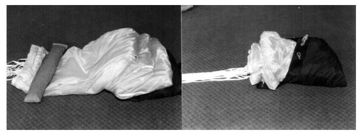
At first make 3 "S" folds on the inner container. Leave the Fold the last 40 cm in small "S" folds in the inner container. last 40 cm without an "S".
