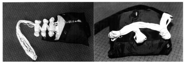
9. Form the lines in 3 "S" forms. The curve on each "S" is loosely secured with rubber bands. The 3 bundles of lines are placed on the parachute.
