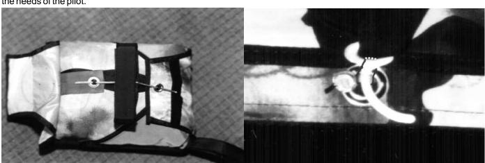
13. Finish by closing the lower fastening flap and finally the 14. To avoid an unintentional opening the DHV prescribe to covering flap.
