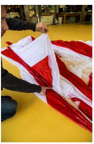
Pic. 64 Put the line attachment point on the middle lines and hold it there
