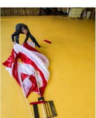
Pic. 78-79 Slide excess material back into the folded panels
