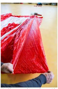
*Pic. 72* Lay panel #4 to the outside and halve it (one fold)
