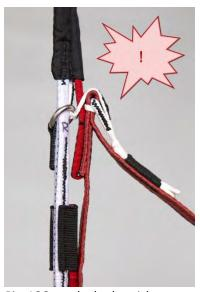
Pic. 15 Pic. 16 Stow the brake stick outside the metal ring!
